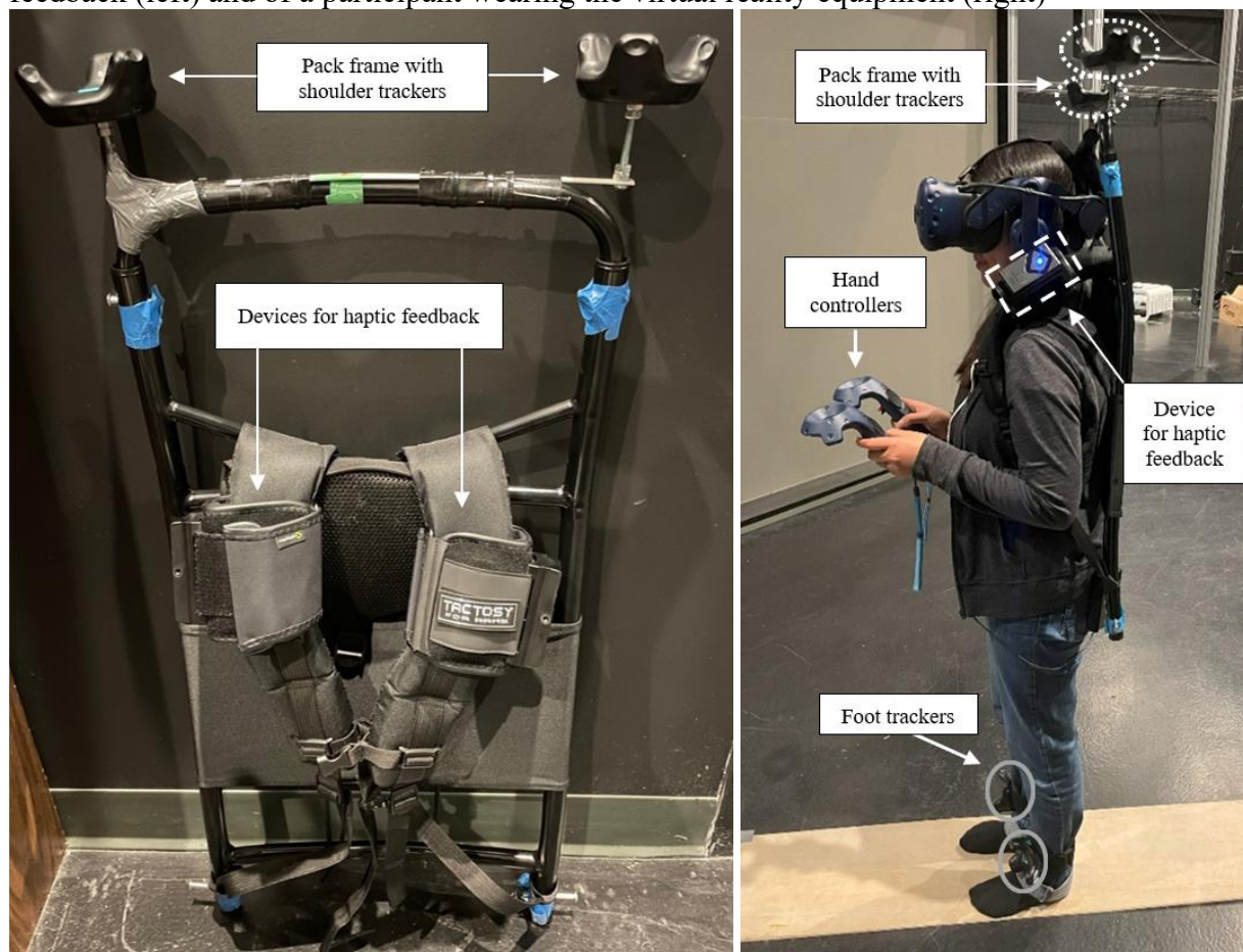
Figure 1 Photo of the devices over the shoulders on the pack frame that delivered haptic feedback (left) and of a participant wearing the virtual reality equipment (right)
