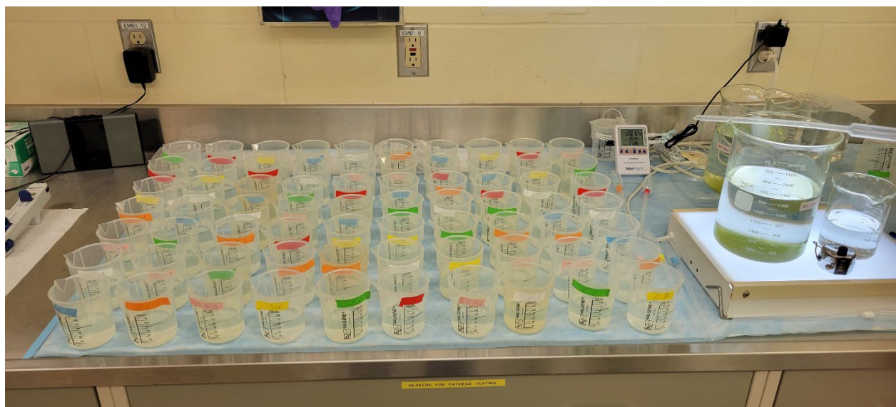
Figure A6. Photograph of the set-up for the toxicity test on Daphnia pulex (water flea). A total of 10 breakers for each lithium treatment ( n=7 ), with one daphnia per beaker.
