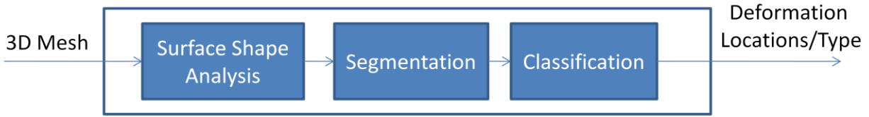
Figure 3.5. System diagram of proposed deformation detection system.
