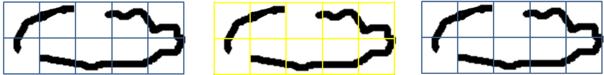
Figure 6.4. Low resolution representation of a feature (Left). Low resolution voxel connectivity shows no discontinuities (Center). Segmentation at low resolution gets entire feature in spite of discontinuities (Right).
