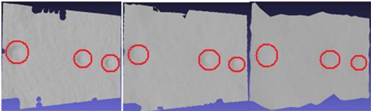
Figure 3.9. Laplacian filtered CPU panel high resolution (Left), medium resolution (Center), low resolution (Right).
