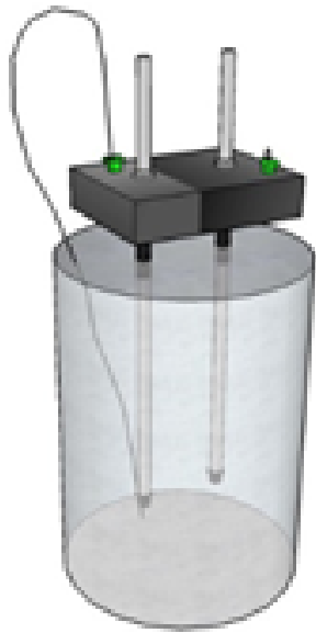
Figure 3.4: Schematic representation and picture of the experimental device used for the measurements of internal resistivity of concrete specimens.
