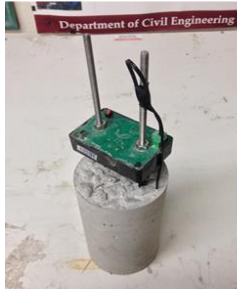
Figure 3.4: Schematic representation and picture of the experimental device used for the measurements of internal resistivity of concrete specimens.
