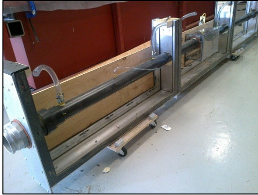
(a) Pressure pipe and feeding hoses
