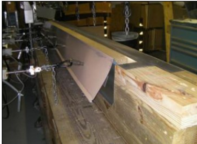
(b) ES-1 test for installed roof edge flashing: failed at 1.87 kPa (39 psf)
