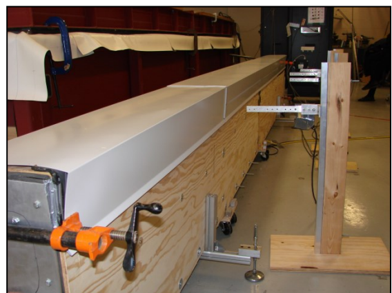
(c) Joining side segment (S-lock)
