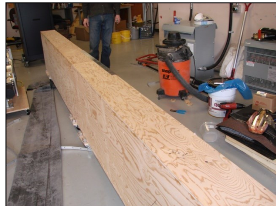
(f) Completed pressure chamber
