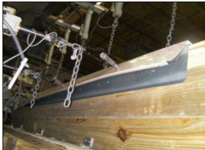
(b) ES-1 test for improved roof edge flashing: failed at 20.6 kPa (430 psf)
