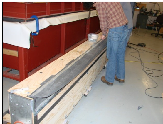
(e) Completed pressure plane
