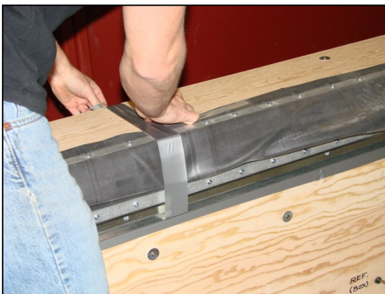
(c) Air sealing the pressure plane
