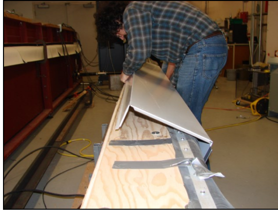
(a) Hooking the coping on the cleat
