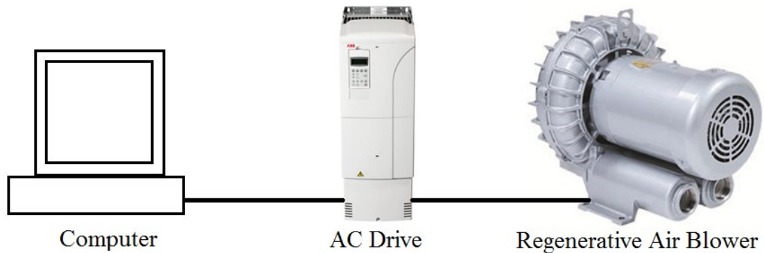
Figure 4.4: Regenerative air blower and AC drive
