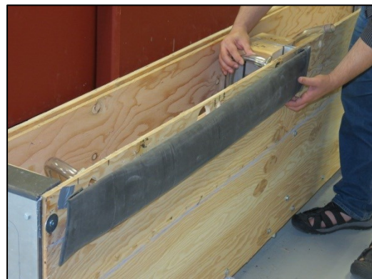
(f) Installation of a pressure bag
