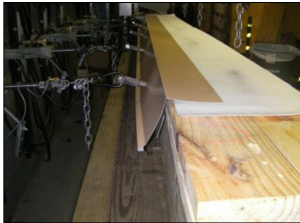
(b) ES-1 test for the installed roof edge flashing
