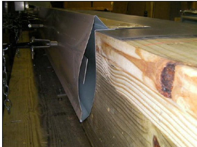
(b) ES-1 test for improved roof edge flashing: failed at 5.50 kPa (115 psf)
