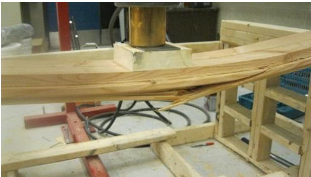
Simple Span 1 Board Failure
