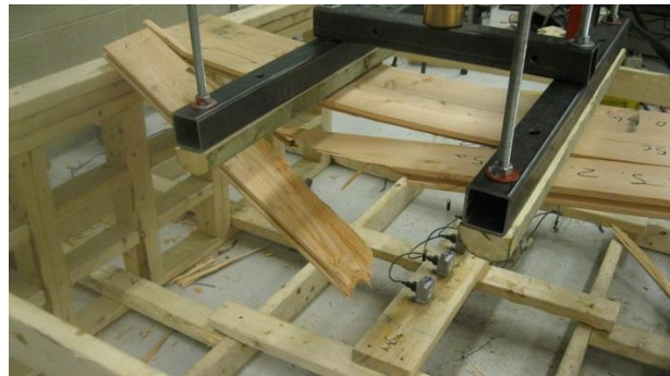
Simple Span 3 Board Failure
