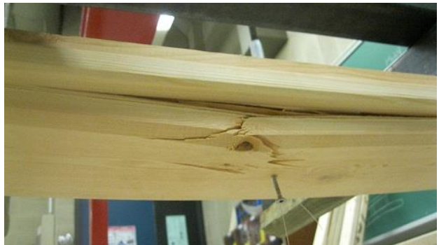
Simple Span 1 Board Failure
