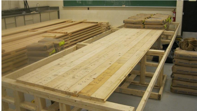
(a) Unbalanced Loading on Span 1 ( 2.42 \text{ kN/m}^2 )
