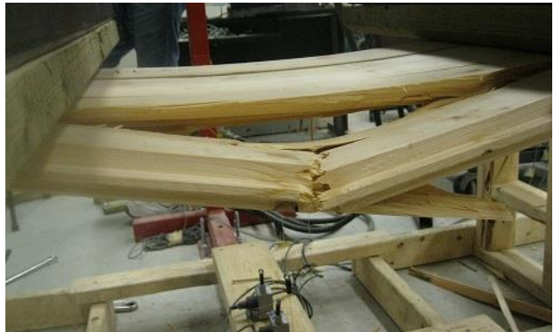
Simple Span 3 Board Failure
