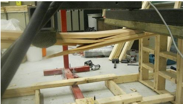
Simple Span 1 Board Failure
