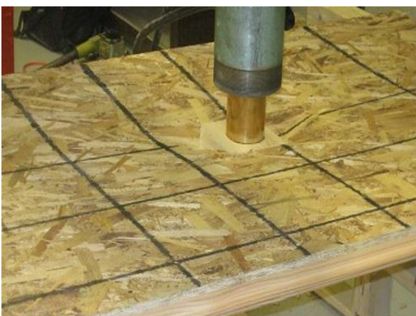
Simple Span 7 Board Failure with sheathing (Top View)
