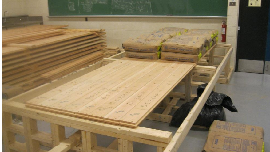
(a) Unbalanced Loading ( 2.42 \text{ kN/m}^2 )
