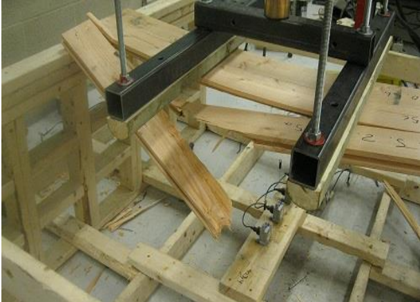
(b) 3 Board Failure
