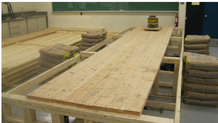
(b) Exterior span of a Controlled Random Layup (1.1 kN)
