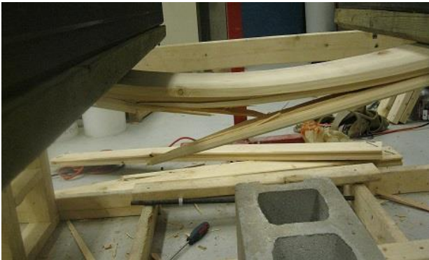
Simple Span 1 Board Failure
