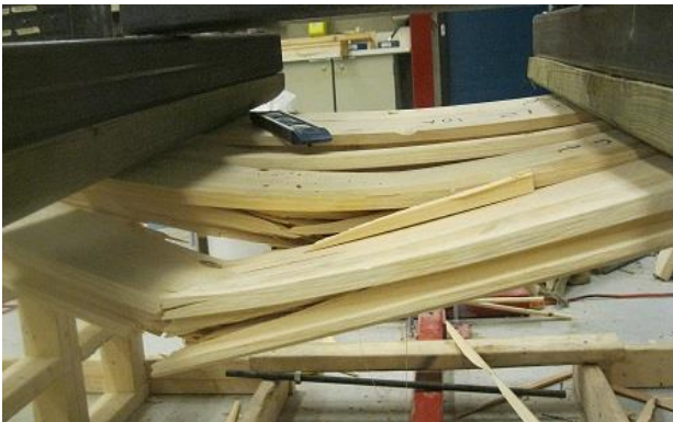
Simple Span 5 Board Failure
