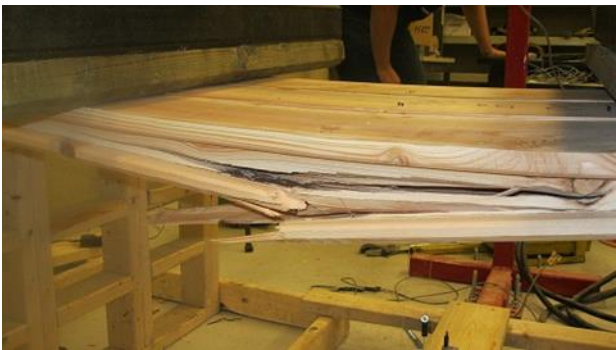
Simple Span 3 Board Failure
