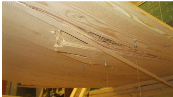
Simple Span 7 Board Failure
