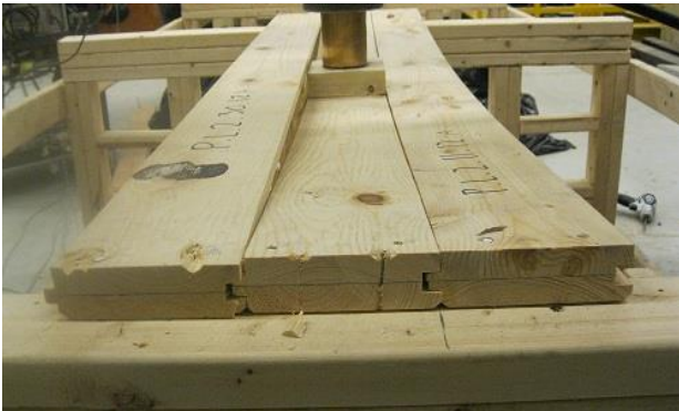
Simple Span 3 Board Failure
