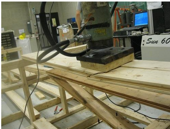
Simple Span 2 Board Failure
