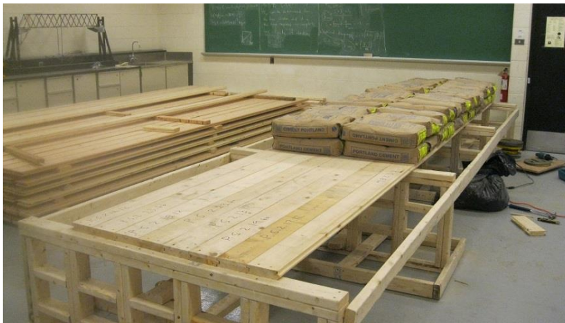
(b) Unbalanced Loading on Spans 1 and 2 ( 2.42 \text{ kN/m}^2 )
