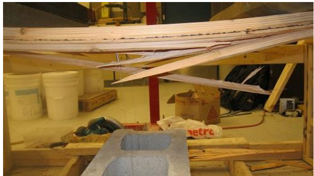
Simple Span 3 Board Failure
