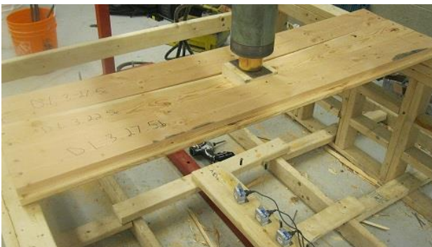
Simple Span 3 Board Failure
