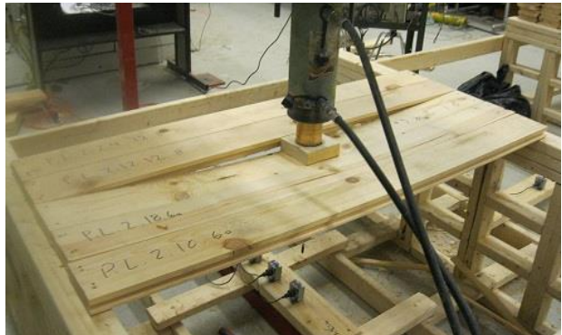
Simple Span 5 Board Failure
