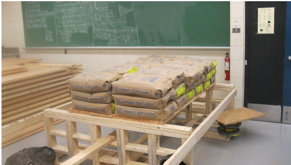
Figure 3.7: Simple Span Layup Non-Destructive Uniform Load Test ( 3.63 \text{ kN/m}^2 )
