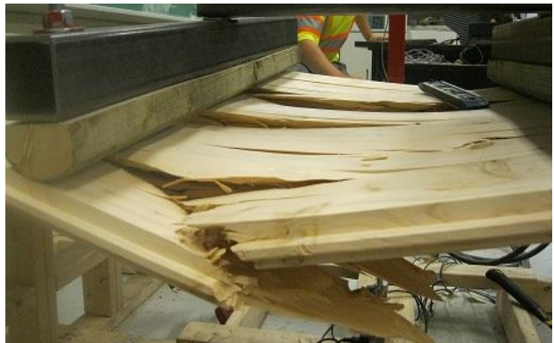
Simple Span 7 Board Failure
