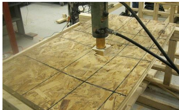
(b) Sheathing Failure
