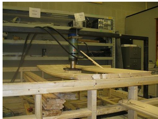
Simple Span 6 Board Failure
