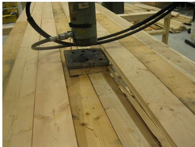
Combination Simple and Two-Span Continuous Failure
