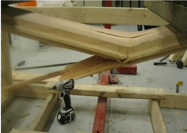
(a) Single Board Failure
