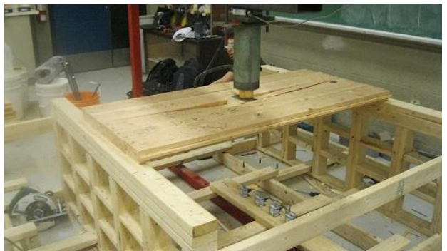
Simple Span 5 Board Failure
