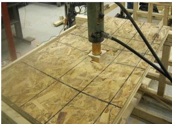
Simple Span 7 Board Failure with Sheathing (Top View)
