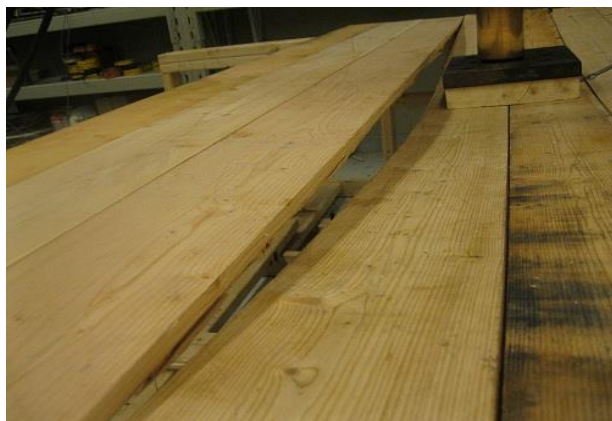
(c) 8 Board Failure (CL200)
