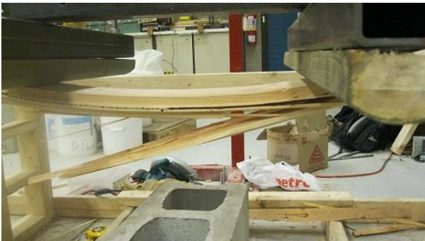
Simple Span 1 Board Failure
