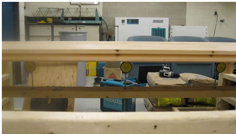
Figure 3.5: Deflection Gauges for Non-Destructive Tests
