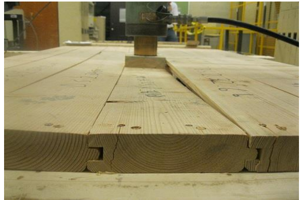
Simple Span 7 Boards Failure
