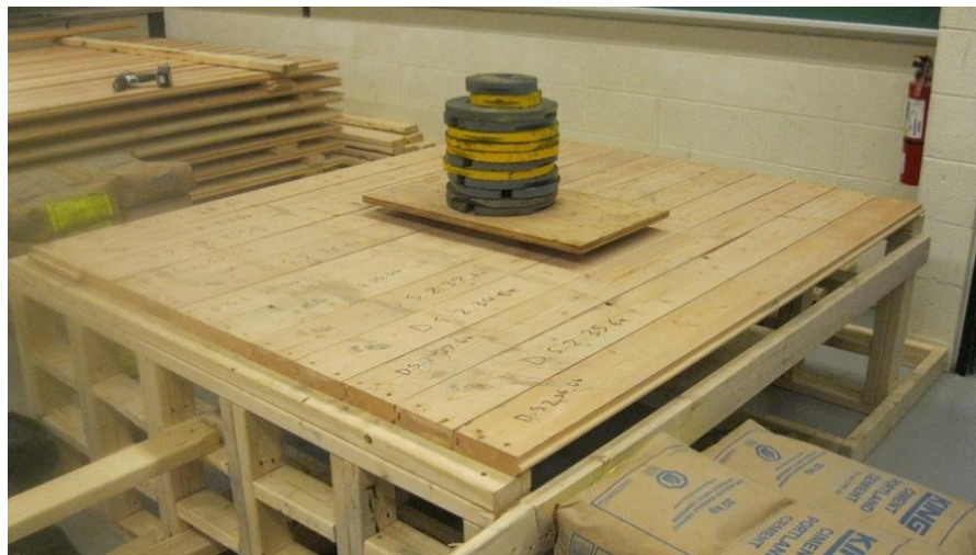
(a) Simple Span Layup (1.1 kN)
