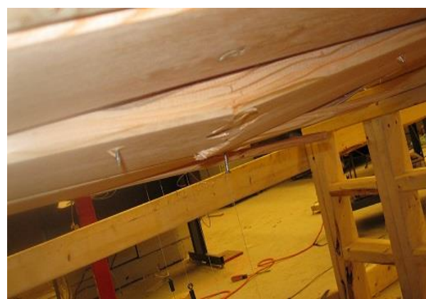
Simple Span 7 Board Failure with Sheathing (Bottom View)
