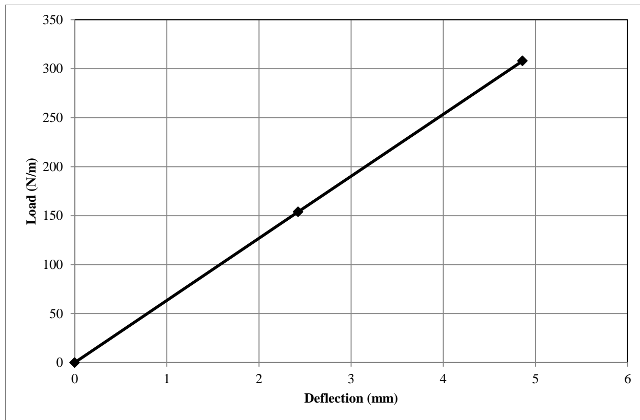
Figure 4.3: UDL vs. Mid-span Deflection Curve – (ND-SS-2-DFL-S2-8)
