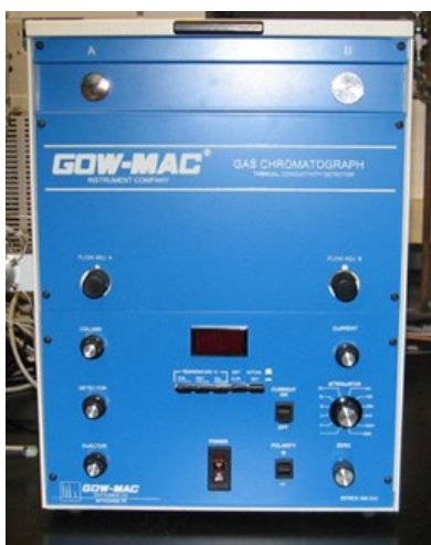
Figure 3-7 GOW- MAC GC Equipment- gases
