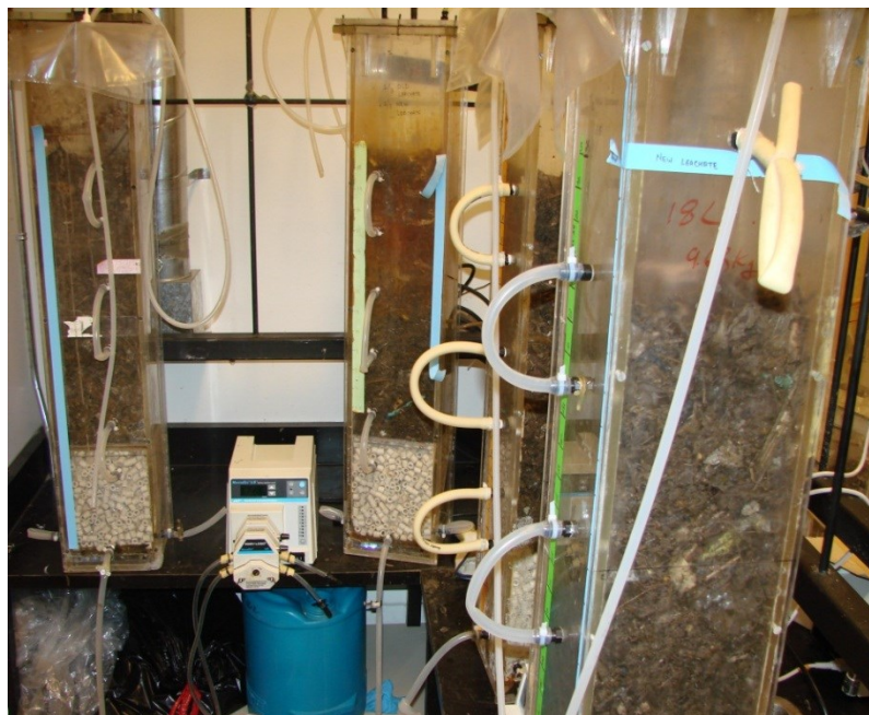
Figure 3-5 Open and closed leachate recirculation loop
