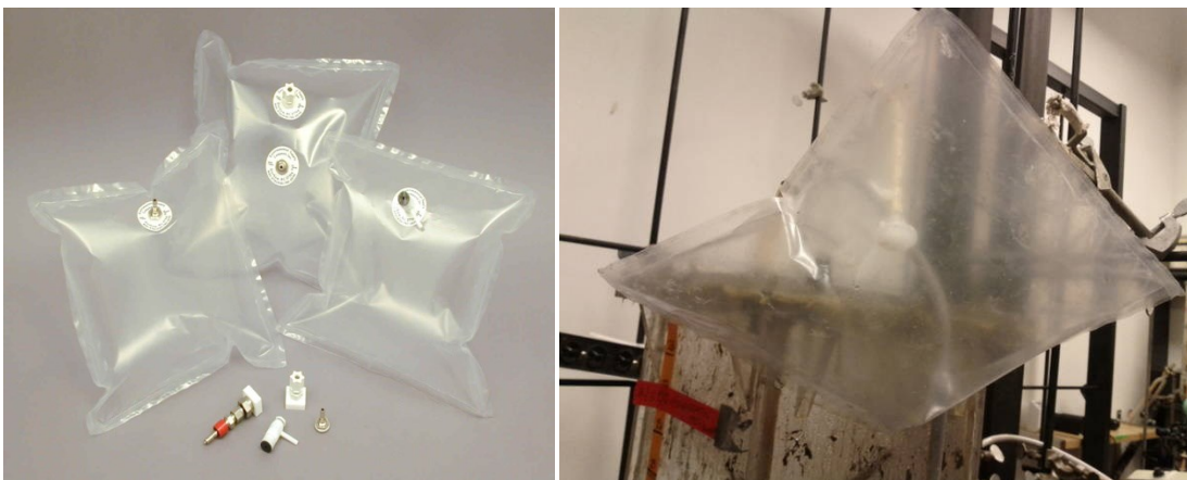
Figure 3-4 Tedlar ® bags for gas measurement
