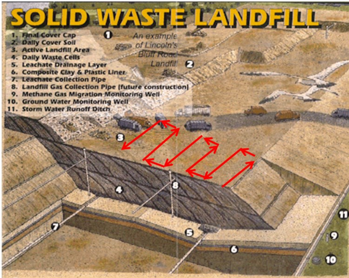
4-25 Landfill loading pattern II-vertical loading (adapted from http://lincoln.ne.gov , (2008))
