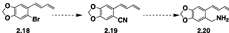
Scheme 2.3: Benzylic amine formation using copper cyanide
