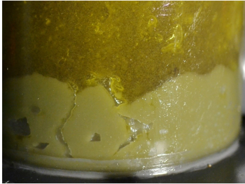
Figure 6.14. Particle sedimentation at U_G \approx 0.25 m/s for a total glycerol concentration of 0.7 wt.%.
