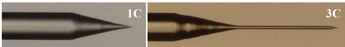
Figure 3.2. 1C and 3C optical probe tips (manufactured by A2 Photonic Sensors).
