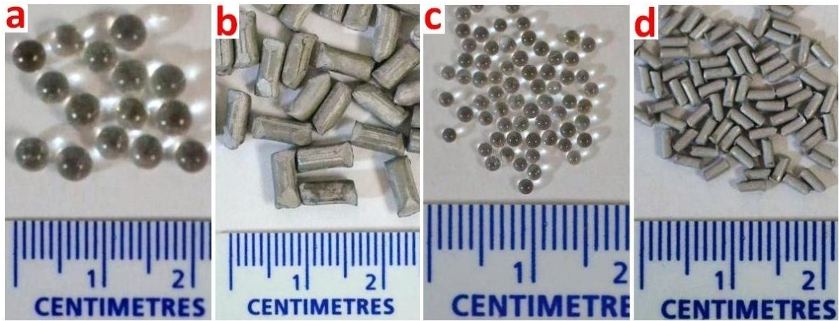
Figure 6.2. Visual comparison of the L spheres (a), L cylinders (b), S spheres (c), and S cylinders (d).
