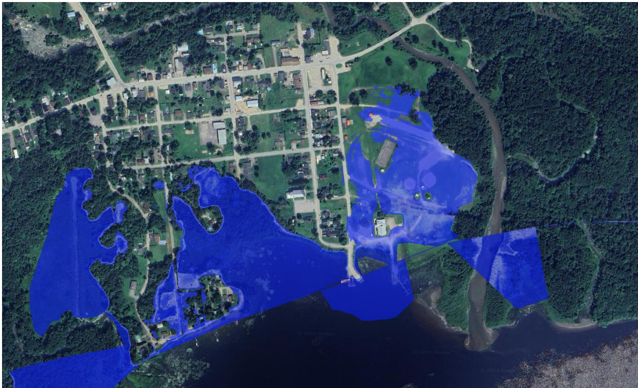
Figure 4.14 - Flood Inundation Map for the 1000-year flood event in the town of Quyón, Quebec.
