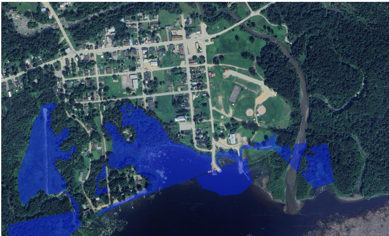
Figure 4.12 - Flood Inundation Map for the 50-year flood event in the town of Quyon, Quebec.
