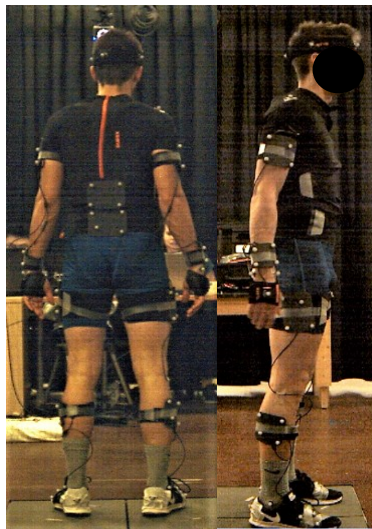
Figure 3.1 Participant setup. A cluster-based optical marker set was worn on top of the Xsens IMU suit.
