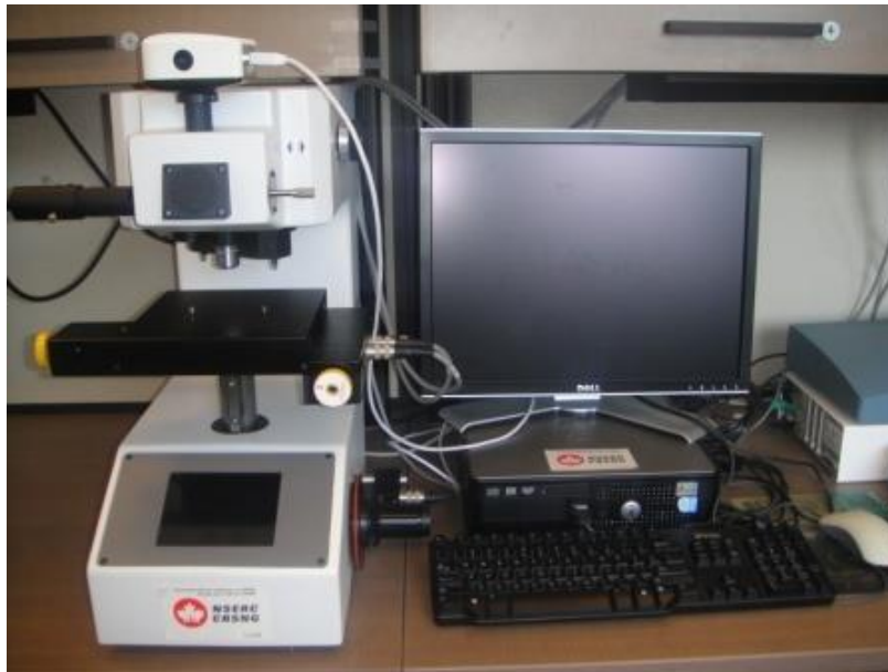
Figure 3-8: Microhardness Tester Unit, Model SMT-X7 Dual Indenter.
