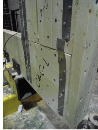
(b) Metal strap failure right face
