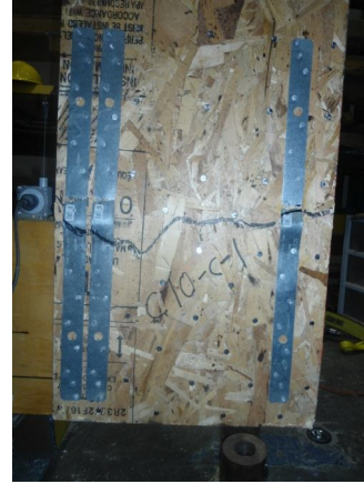
(b) OSB and metal strap failure right face
