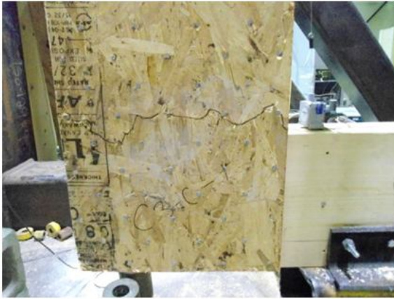
(a) Rupture of OSB left face
