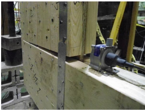
(a) Metal strap failure left face
