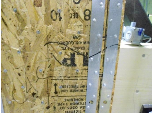
(a) Rupture of OSB left face
