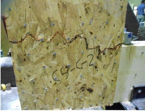
(a) Rupture of OSB left face
