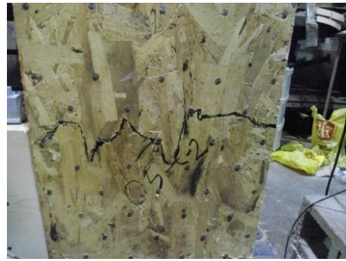
(b) Rupture of OSB right face
