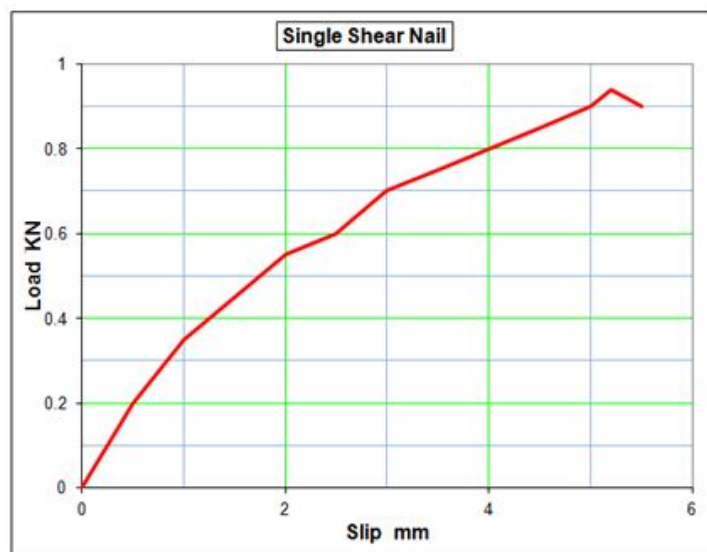
Figure 5.2: Load-slip curve of sheathing to SPF framing nail connection
