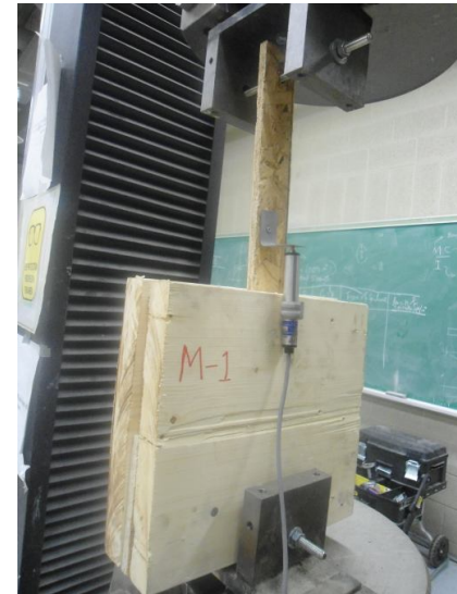
Figure 3.13: (a) Specimen details and (b) actual test setup of double shear nail connection joint.
