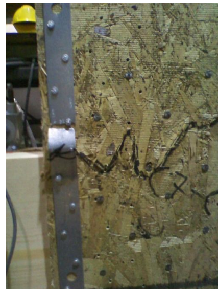
Figure 4.2: Typical failure in sheathing panels for the MIDPLY corner joints.
