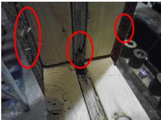
Figure 4.2: Typical failure in sheathing panels for the MIDPLY corner joints.
