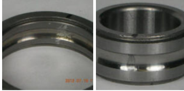
Figure 32: Inner race and outer race faults on the bearings captured by the MFPT dataset [93].
