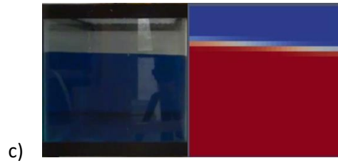
Figure 4- 26 Comparison of free surface in experimental (left) and numerical (right) studies in tank 1 with 200 mm of water, 30° orientation and frequency of lower than resonance
