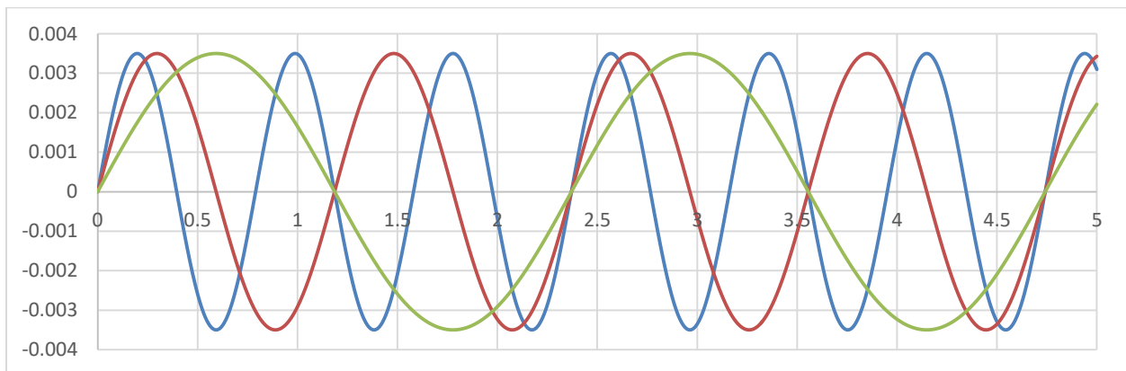
Figure 3- 8 Displacement time history for harmonic excitations of tank 1, water depth 200 mm
