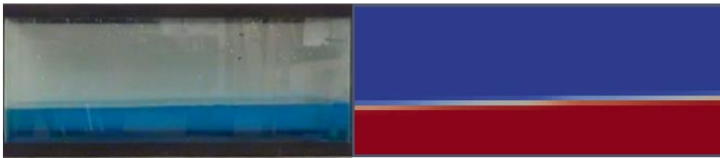
Figure 4- 17 Comparison of free surface in experimental (left) and numerical (right) studies in tank 1 with 100 mm of water, 60° orientation and frequency of lower than resonance
