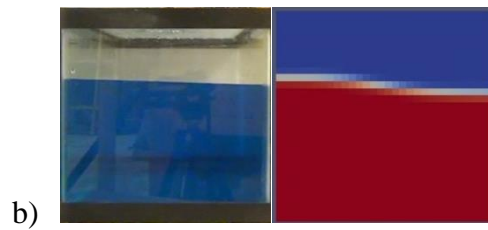
Figure 4- 29 Comparison of free surface in experimental (left) and numerical (right) studies in tank 1 with 200 mm of water, 60° orientation and frequency of lower than resonance
