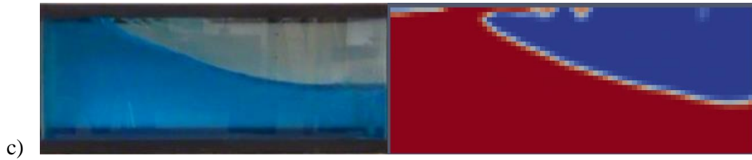
Figure 4- 28 Comparison of free surface in experimental (left) and numerical (right) studies in tank 1 with 200 mm of water, 60° orientation and resonance frequency
