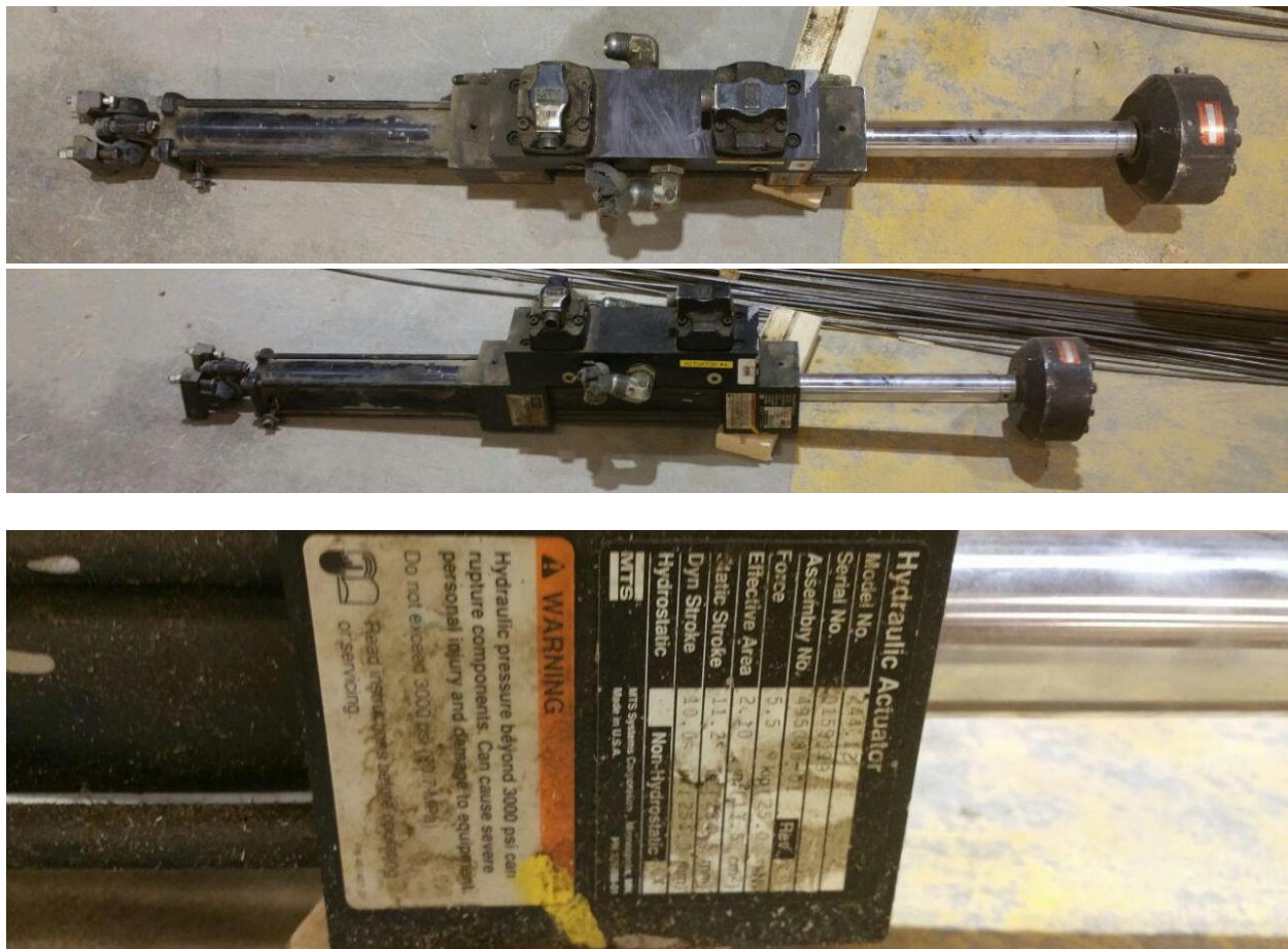
Figure 3- 1 Shaking table actuator from different views
