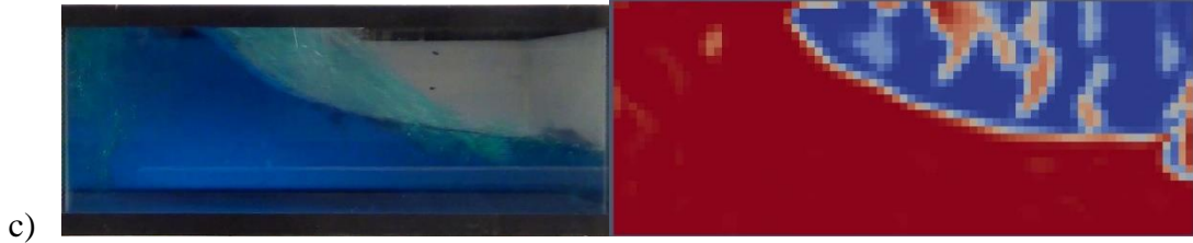
Figure 4- 22 Comparison of free surface in experimental (left) and numerical (right) studies in tank 1 with 200 mm of water, 0^\circ orientation and resonance frequency
