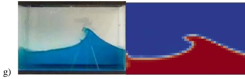
Figure 4- 34 Comparison of free surface in experimental (left) and numerical (right) studies in tank 2 with 100 mm of water, 0^\circ orientation and frequency of higher than resonance
