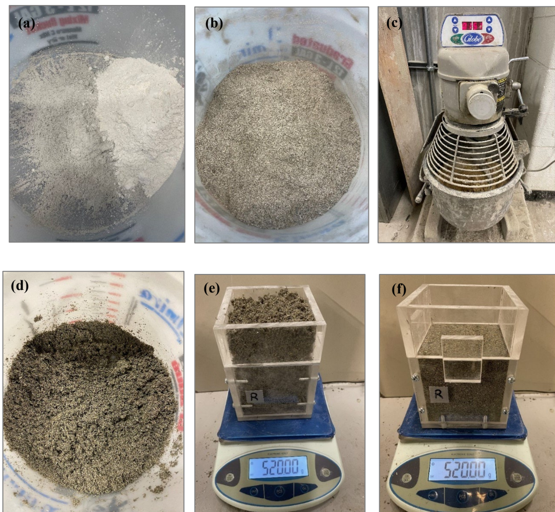
Figure 10- a) Binder components, b) Binder combination with hemp hurd, c) Hempcrete mixture in the mechanical mixer, d) Evenly distributed final mixture, e) Overloading hempcrete in mould, f) Uniformly slight compaction of hempcrete to the mould height.
