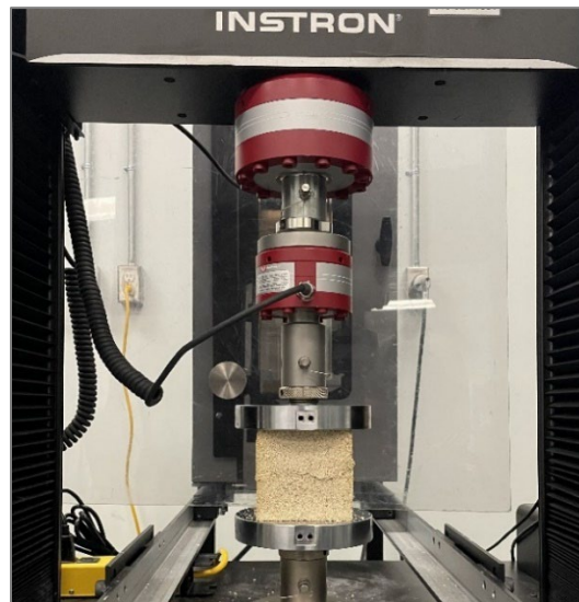
Figure 19- Hempcrete cubes' Compressive strength test
