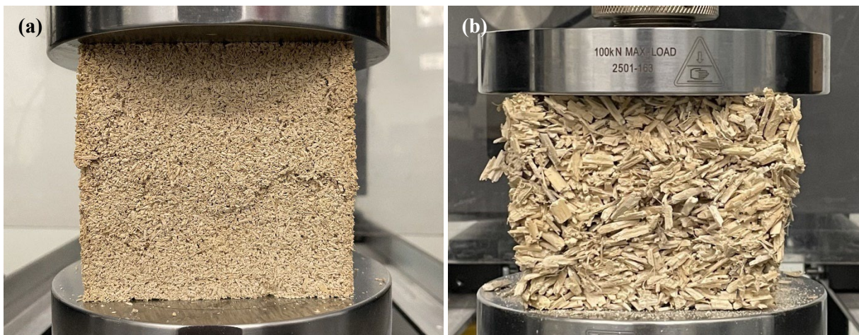
Figure 30- a) The crack in the finely ground hemp hurd hempcrete sample at failure during the compressive strength test, b) The significant deformation in the as-received hemp hurd hempcrete sample without major failure
