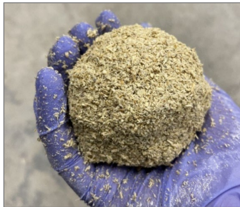
Figure 18- Ball and finger test to determine water demand
