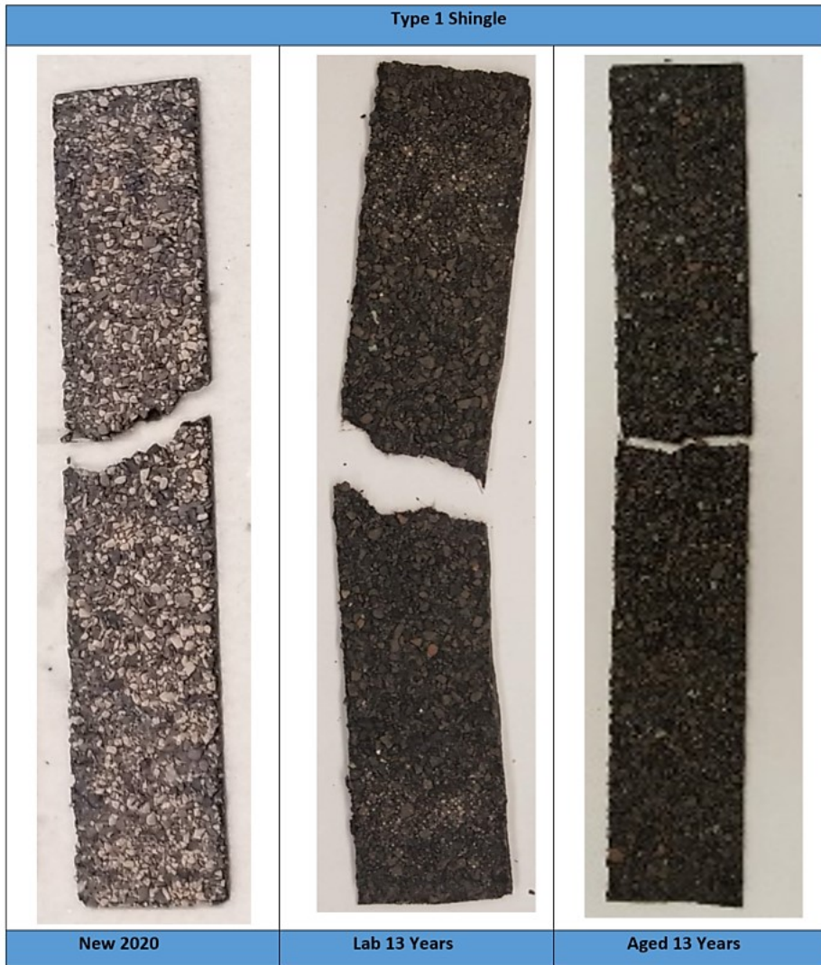
Figure 5.3. Type 1 tensile strength failure modes for MD direction
