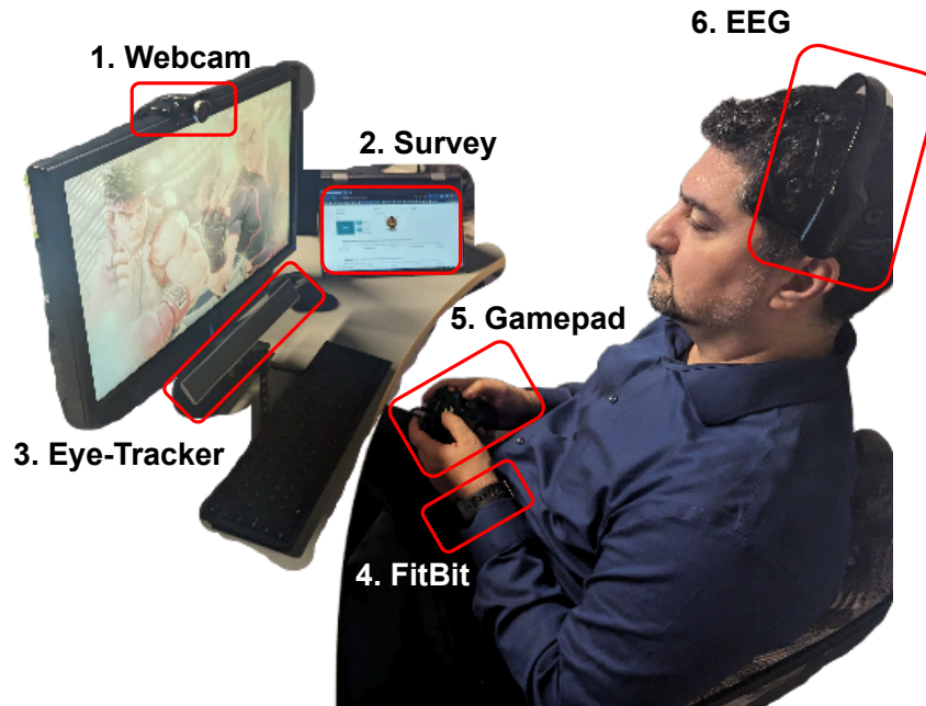
Figure 3.1: Experimental setup showing the integrated hardware components: (1) webcam, (2) survey tablet, (3) eye tracker, (4) smartwatch, (5) gamepad, and (6) EEG headset. ©ACM reused with permission from [15] / cropped and horizontally flipped from original and annotated.
