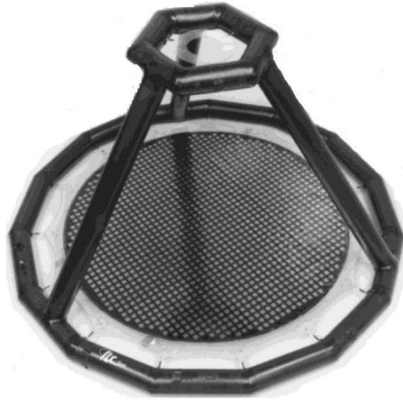
Figure 2.8: 1-m X-band inflatable microstrip reflectarray with circular polarization. (After [31]).
