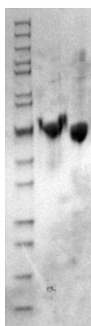
Figure S2. SDS-PAGE analysis of purified recombinant Rad TE and Zea TE. Expected molecular weights are 47kDa and 45kDa. Left to Right: Fischer Rec-Protein ladder (50kDa reference band) , Rad TE, Zea TE.
