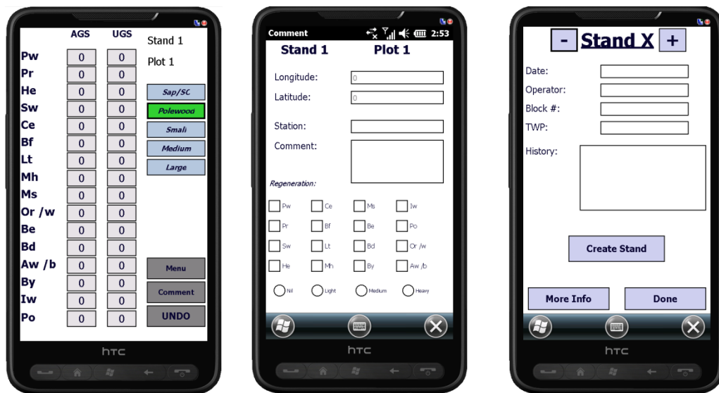
Figure 1.3 Forest stand tally application. The application allows users to electronically enter and record counts of tree information directly on to the mobile device. Data can then be exported into the desktop PC for automated data entry and analysis in MS Excel.
