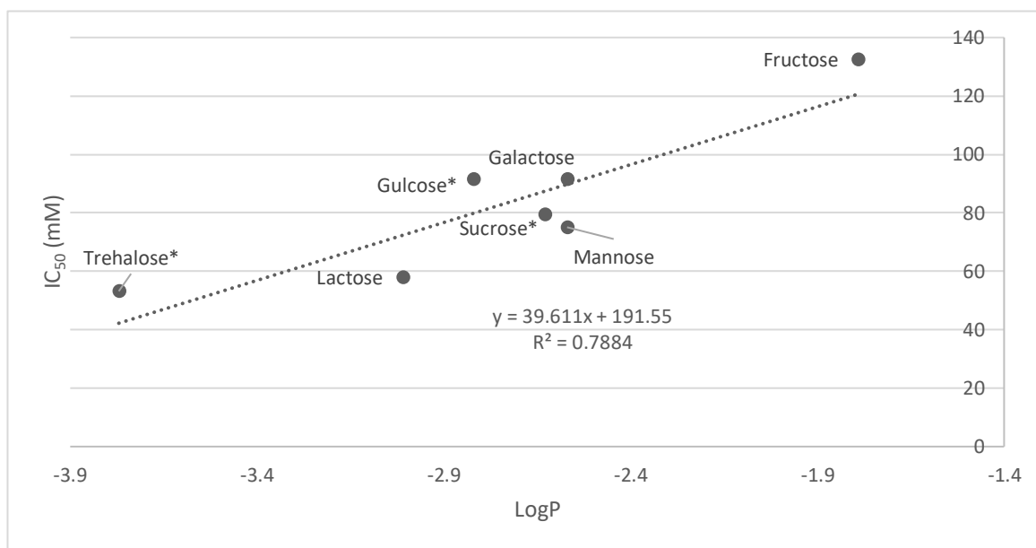
Figure 2.10 - Correlation of LogP calculated using VCCLab's ALOGPS 2.1 to IRI activity (IC 50 ) of monosaccharides and disaccharides using experimental values for D-glucose, trehalose, and sucrose. Experimental values are indicated by *.
