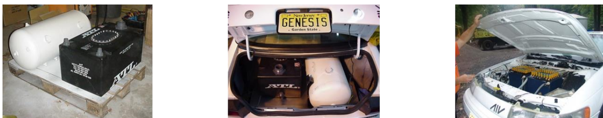
Figure 1.9. First sodium borohydride fueled car designed by Millennium Cell, NJ.
