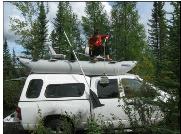
e) Off-lake demonstration of how the Eckman Grab would be used on the lake. Photo by Carley Crann.
