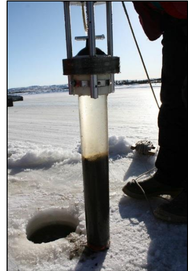
c) Glew core barrel with sediments extracted from the top 30 cm of lake-bottom sediment. Photo by Jennifer Galloway.
