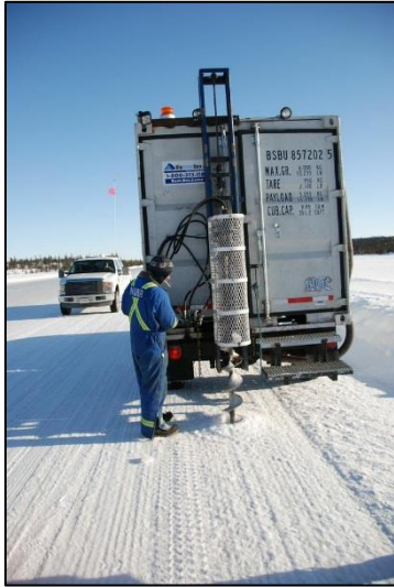
a) Truck with rear-mounted auger used for drilling holes in the ice along the Tibbitt to Contwoyo Winter Road. Photo by Jennifer Galloway.
