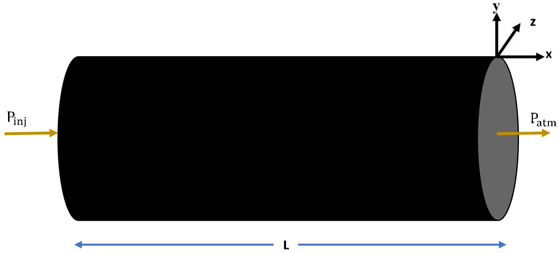
Figure A1. 1D Gas Flow through a porous medium of length, L.
