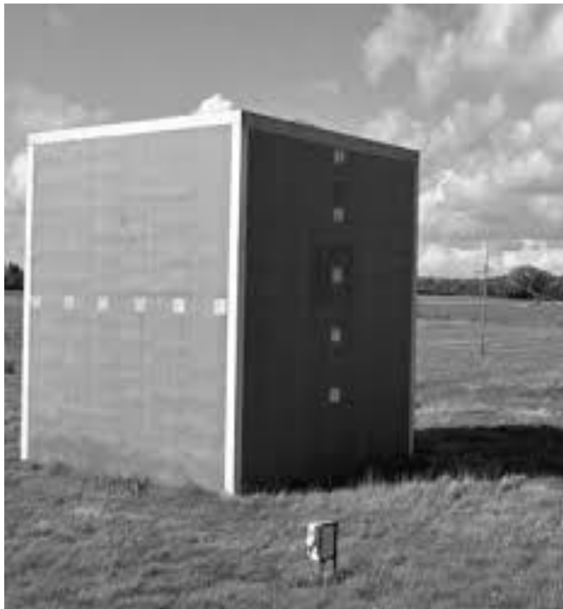
Figure 2. 7 The full-scale Silsoe Cube building (Richard and Hoxey, 2012)
