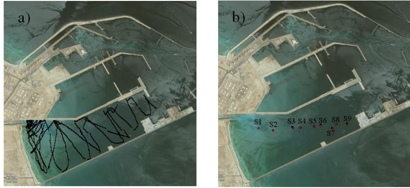
Figure 5.5: a) The survey path; and b) the location of the stationary measurements for vertical temperature profiles
