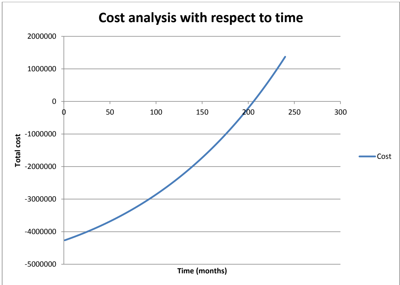
Figure4.3: Total cost versus time (months) for a total drilling length of 10,000m
