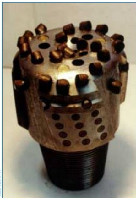
Figure1.9: Diamond cutter drill bit [21]
