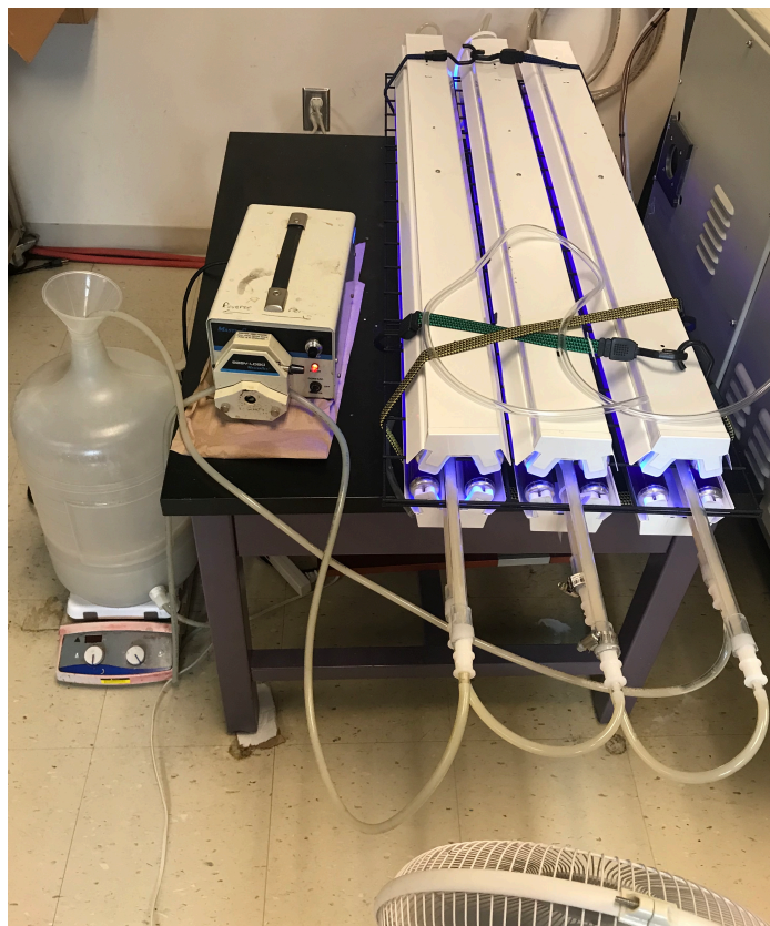
Figure 4.4. Similar set up of scaled- up reaction for the large batch synthesis of Hinton A lignin@TiO 2 nanoparticles irradiated with UVA light from 3 stations, each with 4x 40 W bulbs.
