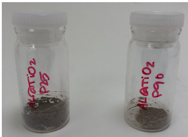
Figure 4.18. Picture of Hinton A lignin@TiO 2 nanoparticles synthesized using P25 (left) and P90 (right) TiO 2 powder.
