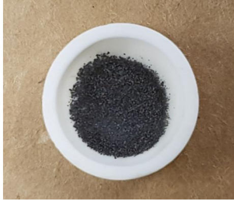
Figure A-5: Sample pan loaded with 40 mg of ilmenite sample
