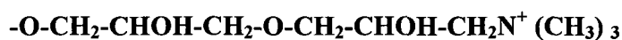
Figure 4.9: Structure of the charged functional moiety present in a mono Q resin
