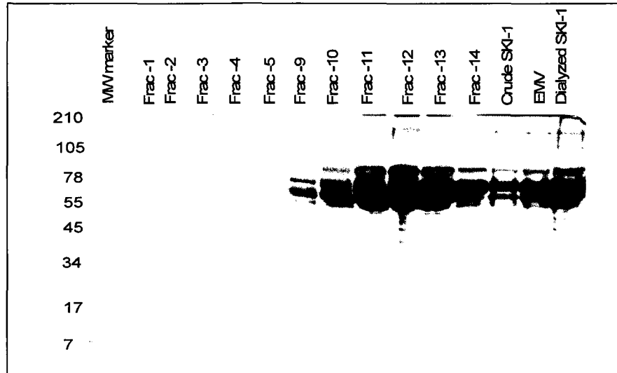
Figure 4.15: 8% Tris tricine SDS-PAGE for the enzymatically active fractions collected during the purification by size exclusion (Superdex 200 10/30GL) chromatography shown in Figure 4.13. Fractions are selected according to the activity profile (Figure 4.14).
