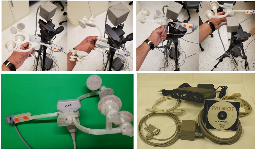
Figure 6-33. Illustration UltraChin connected to Electromagnetic Sensor. The receiver of the Electromagnetic tracker is attached to the camera. ProbeNet tracks the upper left corners of the two orange squared markers for the calculation of transformational information. The electromagnetic tracker is Polhemus Patriot TM. First row: different views of magnetic tracking sensors attached to UltraChin. Second row: Different parts of UltraChin and magnetic tracking sensor can be seen in the figure.
