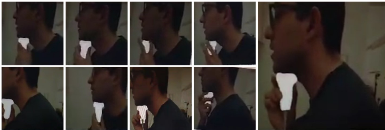
Figure 4-6. Randomly selected frames for the evaluation of real-time probe segmentation using the sU-NET deep learning model.
