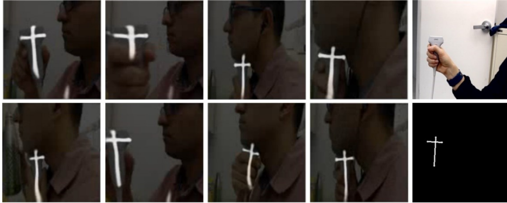
Figure 4-8. Sample frames from real-time testing the sU-NET for segmentation of the probe for localization.
