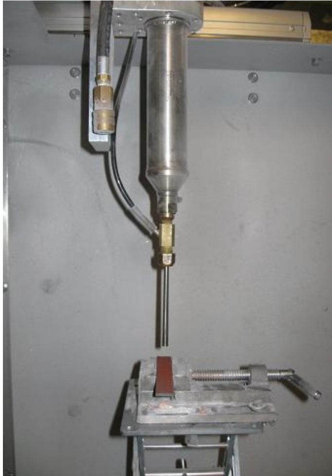
Figure 3.22: Inside the LP-CGDS spraying chamber
