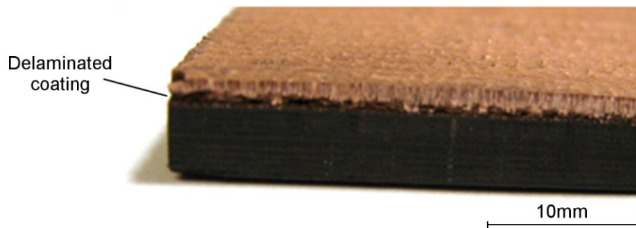
Figure 5.6: Coating delamination in one corner of the IHCT-CPMC
