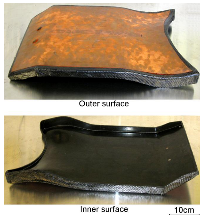
Figure 1.1: Backseat integrally heated composite tooling (IHCT) designed by NRC-IAR [4]
