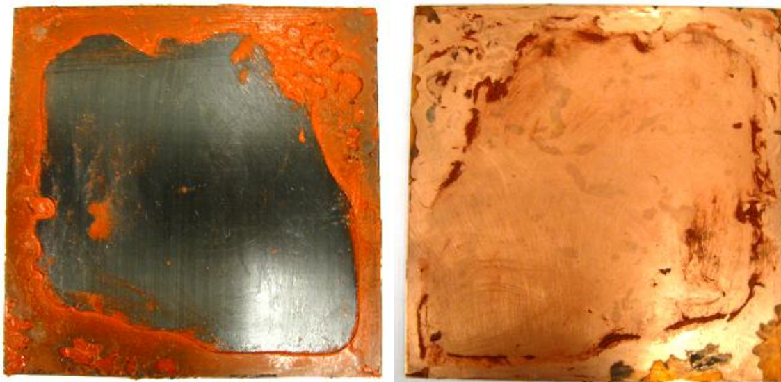
Figure 5.21: PMC plate with cured silicone (left) and copper sheet with cured silicone (right) of the IHCT-NRC #1 after disassembly where the uncured silicone was cleaned before taking pictures
