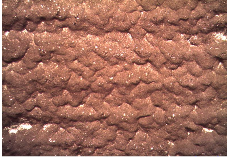
Figure 4.13: Microscopic image of the coating surface where particle splats are observed
