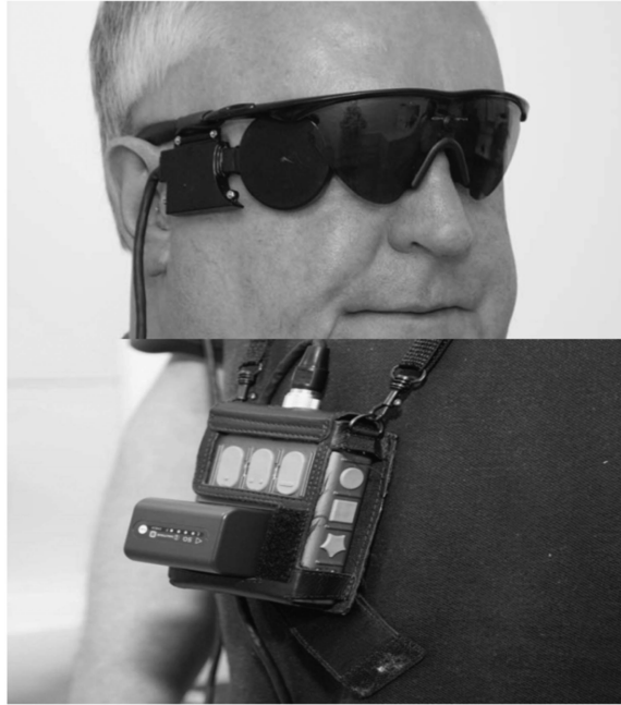
Figure 2.3: Argus II external system consist of a camera mounted on a glasses frame along with the power and data induction coil. Power and information is provided by an external waist mounted unit.
