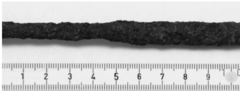
Figure 2.4: Uniform corrosion (reproduced from Angst et al., 2012), (ruler's unit: cm)
