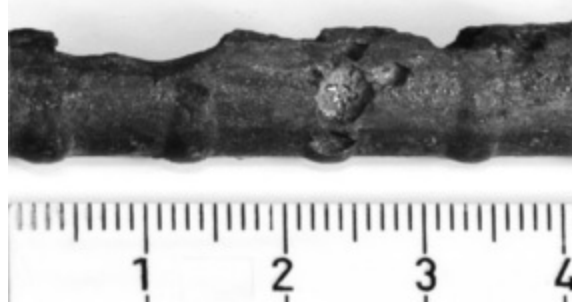
Figure 2.6: Localized corrosion (reproduced from Angst et al., 2012), (ruler unit: cm)
