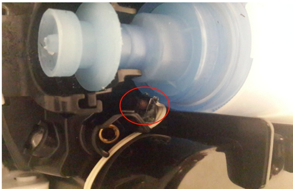
Figure 14 Momentary switch (in the red cycle) placed inside the intelligent dispenser
