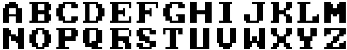
Fig. 4.30. The task set used to consist of 26 binary input vectors of 100 dimensions shown in 10 by 10 format, where black pixels represent the value of 1 and white pixels the value of zero.
