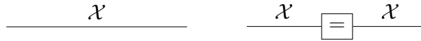
Figure 2.3: Equality Insertion/Deletion Procedure. Left to right: Equality Insertion; right to left: Equality Deletion. The edges may be regular or dangling; the vertex labelled with “=” represents the function \delta_=_ .
