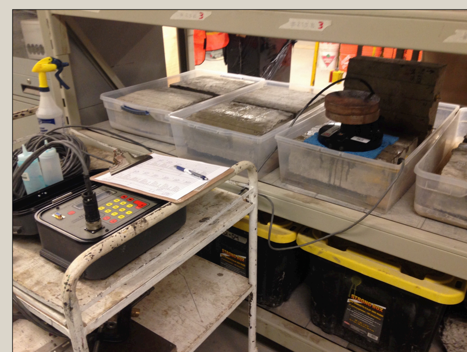
Fig. 3: Corrosion rate testing with the Gecor sensor.
