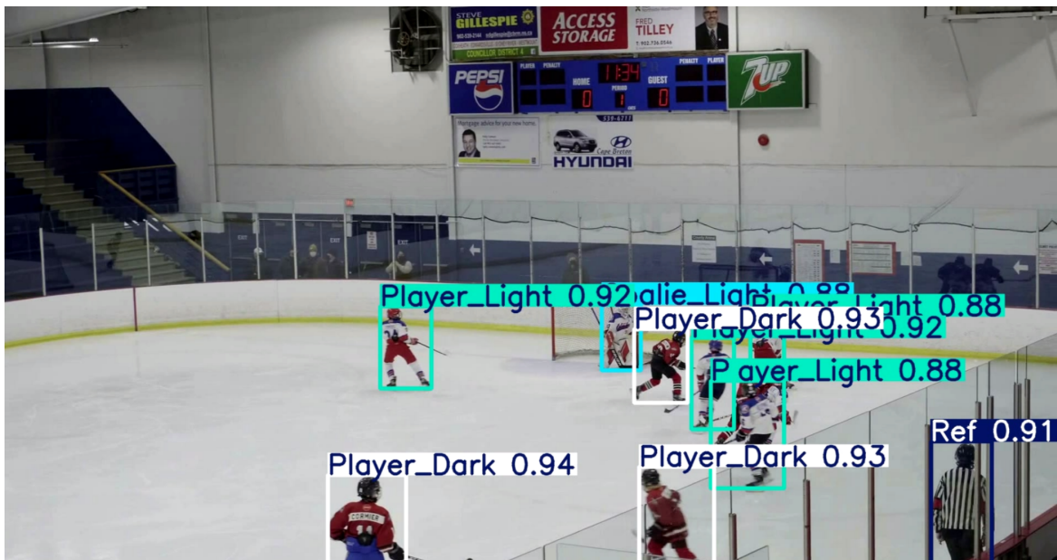
Fig. 5.2 Player detection results showing the five-class labeling strategy with confidence scores. The system successfully distinguishes between Player_Light, Player_Dark, Goalie_Light, Goalie_Dark, and Referee classes, enabling robust tracking even in crowded scenarios. Confidence scores above 0.4 indicate reliable detections.
