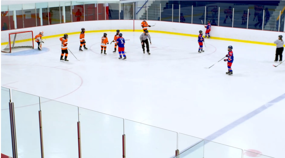
Fig. 1.3 Example from youth hockey video illustrating typical technical challenges. At this camera distance, players appear extremely small with heads occupying fewer than 30 pixels, making precise impact detection difficult, particularly under motion blur and partial occlusion near the boards.
