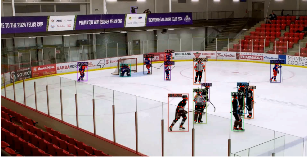
Fig. 2.6 Appearance-assisted tracking preserves identity (colour-coded boxes) as two skaters collide and separate.
