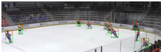
(a) Undetected head impact due to player occlusion. Head detection fails when players are in close proximity.
