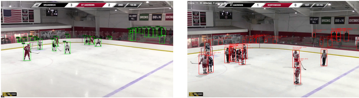
Fig. 5.3 Player tracking performance comparison. Left: Successful multi-object tracking with stable ID assignments during normal gameplay, showing consistent identity maintenance across multiple players. Right: Tracking failures during crowded scenarios with detection overlaps and missed assignments, illustrating the challenges that contributed to Model A's degraded performance.
