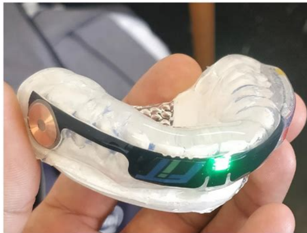
Fig. 2.2 Commercial instrumented mouthguard (Jones et al. , 2023). The on-board tri-axial accelerometer, gyroscope, and Bluetooth radio are embedded in a rigid dental shell, yielding high-fidelity skull kinematics.
