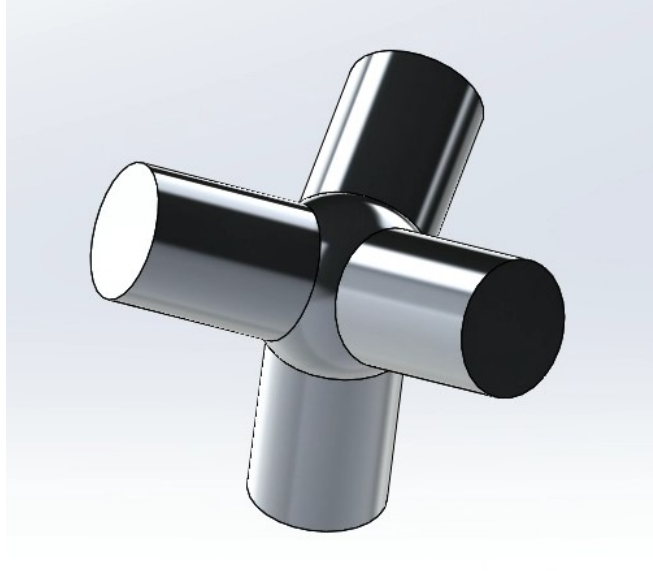
Figure 9.1 Tetrahedral shape consisting of a node with four arms at 109.5^\circ from each other. The arms are 0.3 mm from the center of the nodes. Made using SolidWorks 2019.
