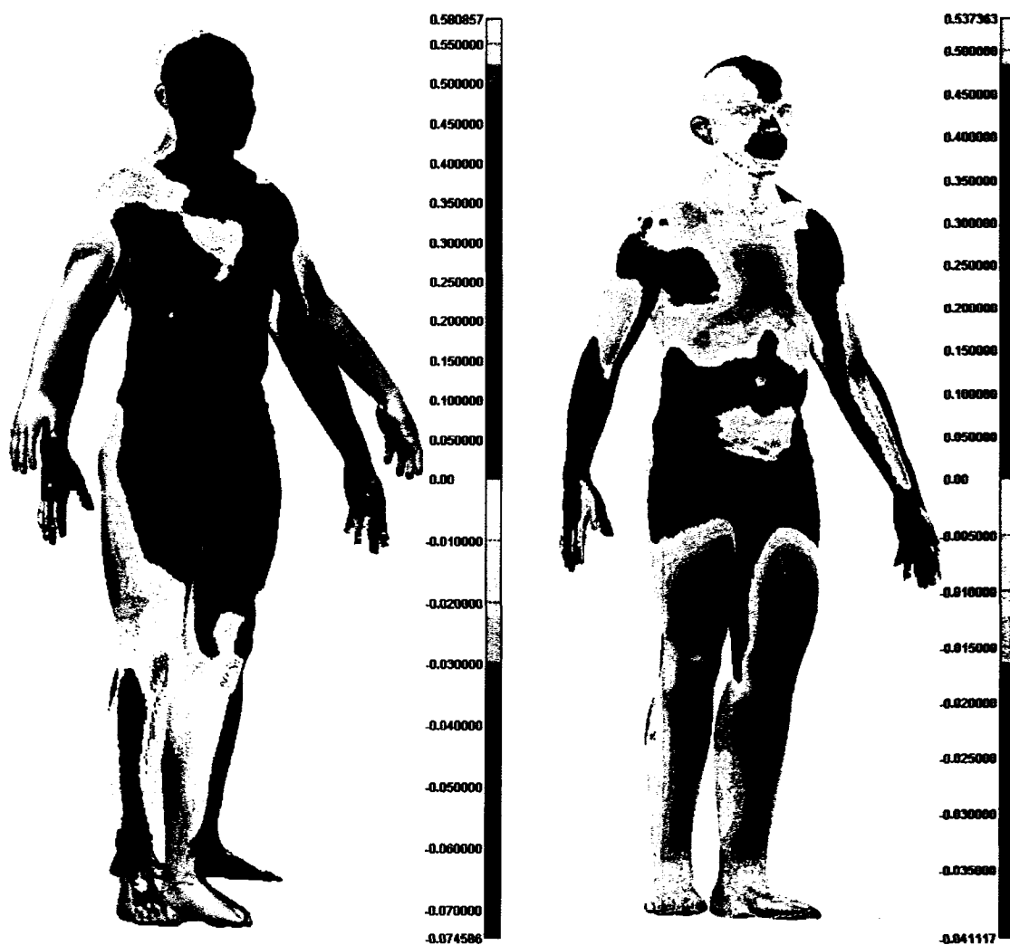
Figure 16: Comparisons between the target “csr0232a” and the generic model (left: original generic model in grey and the target, right: RBF-deformed generic model and the target)
