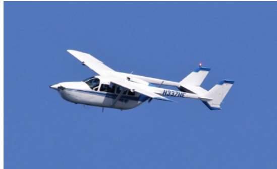
Figure 2.7: The Cessna 337 Skymaster used by the Center for Coastal Studies to conduct aerial surveys in Cape Cod Bay in 2021. Note the distinct twin tail design. Photo from CCS Facebook page accessed 29 August 2025.
