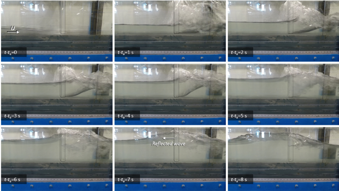
Figure 43. Bore impact on column and wave reflection causes water level rise at front of column (test D40-S520)
