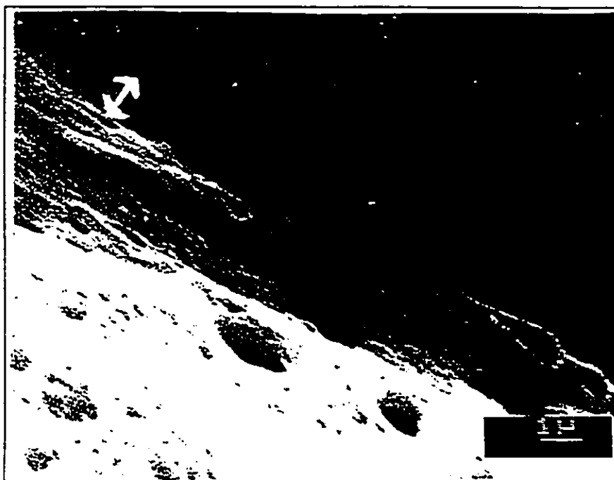
Figure 6.10 Scanning electron micrograph of a cross-section of membrane 6-15C-6-5, the skin layer is indicated by the arrow.
