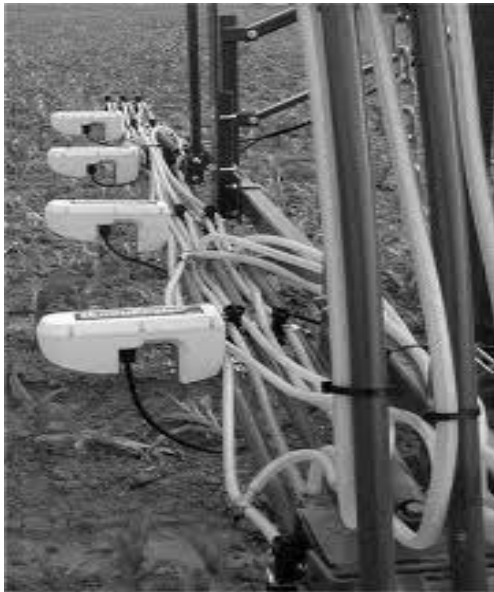
Figure 2.1. Greenseeker sensor: a) Capture of information. b) Tractor-mounted sensors on-the-go (Source: NTech Industries, Inc)
