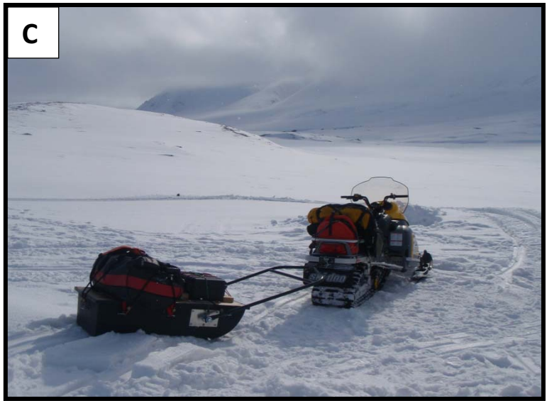
Figure 3.17: Ground penetrating radar field set-up. (A) 50MHz GPR system custom fitted onto a komatiq; (B) Custom fitting 250 MHz GPR into plastic sled; (C) GPR sled pulled behind a skidoo. Photos: Luke Copland (A&B), Colleen Mortimer (C).
