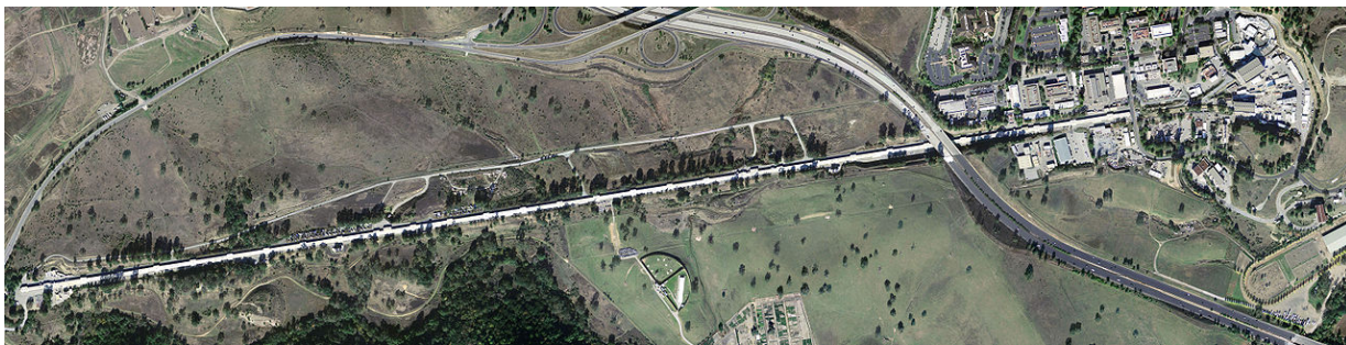
Figure 1.3: Birds eye view of the Linac Coherent Light Source (LCLS). The instrument was converted from the existing linear accelerator at Stanford Linear Accelerator Center (SLAC) and it achieved first lasing in April 2009. The source is capable of producing a trillion X-ray photons per pulse, at 100 femtosecond pulse duration. The picture shows the 2 mile long linear accelerator [11].
