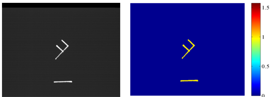
Figure 5.1: The sample used in the simulation is a bit map converted from a real sample. The picture on the left is taken from a light microscope. The length of the reference slit is on the order of 20 \mu\text{m} . The picture on the right shows the converted bit map. We use the picture on the right as our diffraction sample and the true object space for all simulation in this section.
