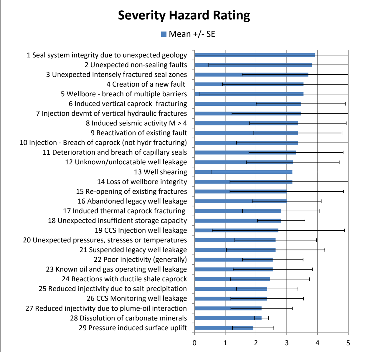
Figure 4.8: Mean expert rating of the severity of twenty-nine potential hazards should they occur, including standard error as a measure of uncertainty in expert opinion. [Ratings range from: light (1); serious (2); major (3); catastrophic (4); multi-Catastrophic (5).]
