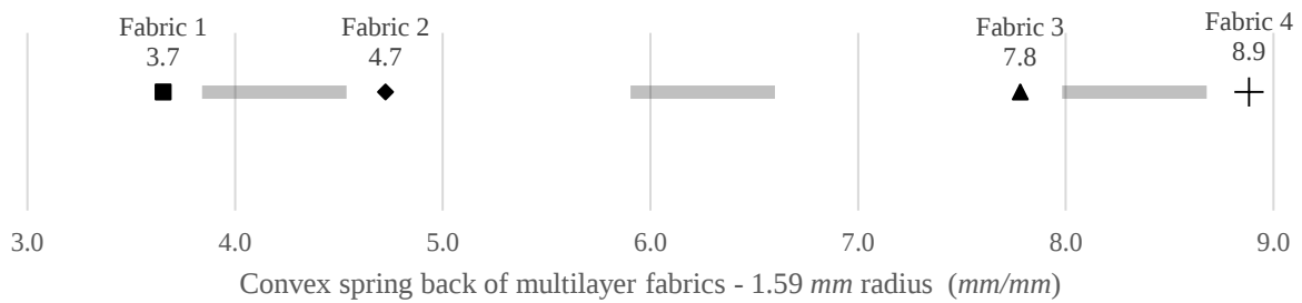
Figure 4.18 – Convex spring back of multilayer fabrics – 1.59 mm (1/16 th in) radius
